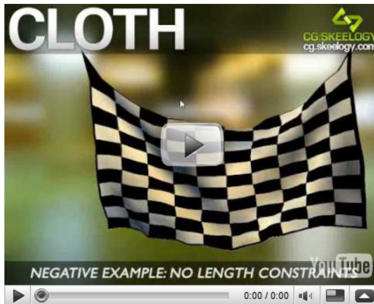
Video 6: A cloth simulation without length constraints. The cloth tends to be too elastic and quite unstable at times. [Click on image above to watch the video]
