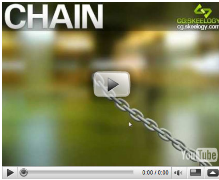
Video 3: An interactive chain simulation (created using springs and length constraints) [Click on image above to watch the video]
