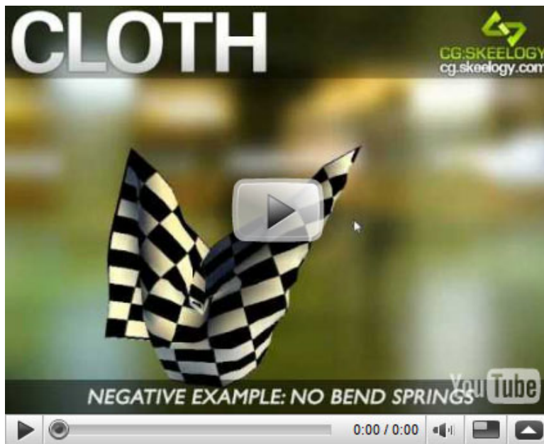
Video 8: Cloth simulation with structural and shear springs (no bend springs). The cloth holds its shape better but is unable to bend realistically and penetrates itself easily. [Click on image above to watch the video]
